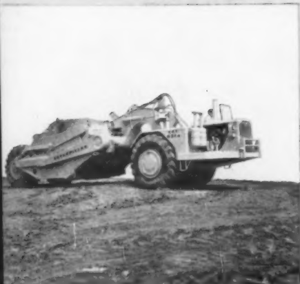
NEW 631 420 HP (335 HP flywheel) . . . 31.2 MPH . . . 28 cu. yd. (21 cu. yd. struck).
